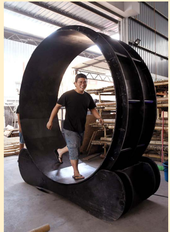
Kong demonstrates the way to generate electric energy through the hamster wheel, which can then be used to charge phones and computers or even power lights.
